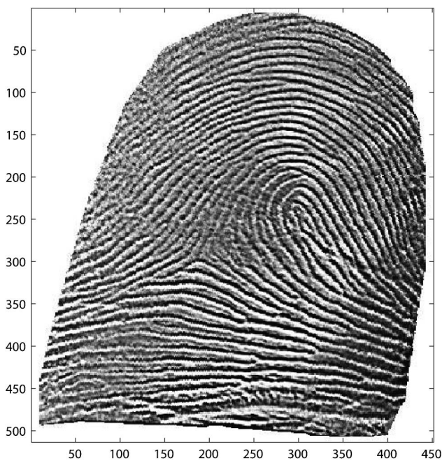
Fig. 7. The final 3D unwrapped fingerprint downsampled to 500 ppi. The width of the resulting image is 450 pixels, and the height is 510 pixels.
