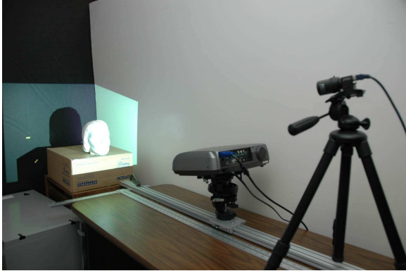
Figure 6. Our experimental setup. A sliding projector is in the middle and a video camera is on the right.
