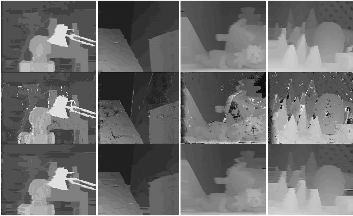
Figure 5. Resulting depth maps from the Middlebury stereo data set. (top row) vertical aggregation (one-pass) + DP; (middle row) two-pass aggregation + WTA; (bottom row) two-pass aggregation + DP
