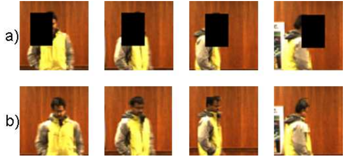
Fig. 7. Inpainting of foreground object with varying pose: a) The first row shows the magnified version of the input sequence with the hole. b) The second row shows a close-up look of the final inpainting results using our algorithm.
