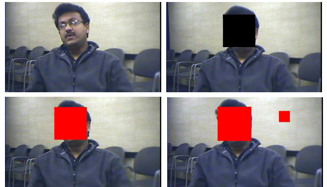
Fig. 4. Top-left: a frame from the original sequence; Top-right: face blocked when the subject is not speaking; Bottom-left: face blocked when the subject is speaking; Bottom-right: false alarms on the background wall.
