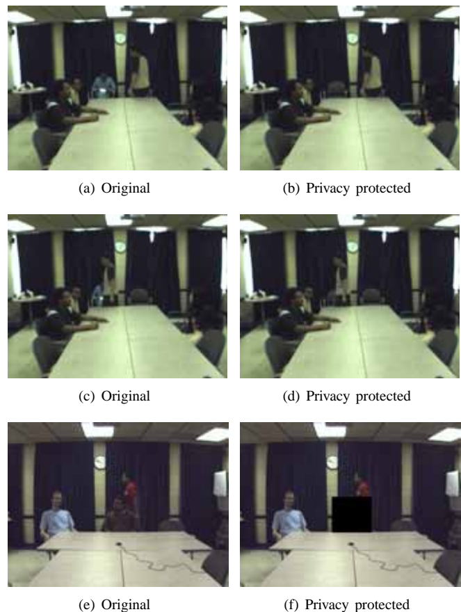
Fig. 4. Privacy protection under both schemas: The first row shows the privacy protection of the unoccluded stationary PPP. The 2nd row shows privacy protection of the partially occluded PPP. The 3rd row shows the privacy protection of the APP by black boxing.
