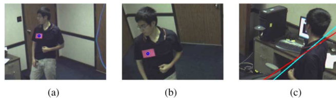
Fig. 1. Tag is visible only in two camera views Cam1 and Cam2 but not in Cam3, but its location in Cam3 can be uniquely determined by the intersection of the two epipolar lines. (a) Cam1 original. (b) Cam2 original. (c) Cam3 epipolar lines.
