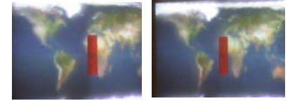
Figure 5: The view-dependent effect of our display. The red cylinder in front of the world map is blocking different parts of Africa.
